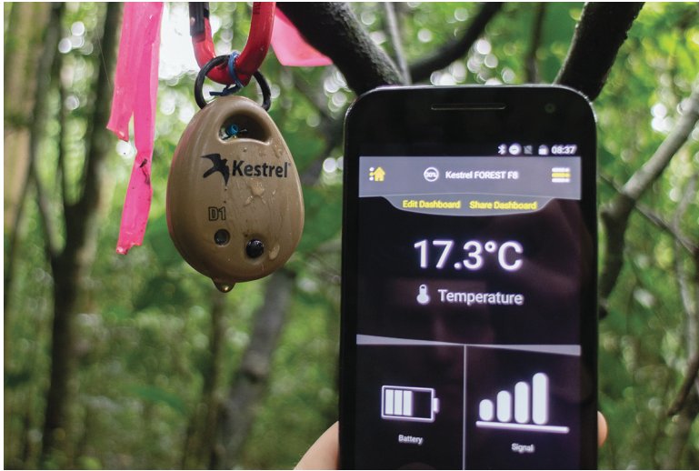
Figure 9.2 Kestrel Drop 1 temperature logger connected wirelessly to a Motorola Moto E (2014) Android smartphone via Bluetooth and the Kestrel LiNK app. Universal standards for Bluetooth and WiFi wireless connectivity mean consumer smartphones and tablets are increasingly compatible with data recording loggers and sensors. In this case, wireless connectivity means the logger can be positioned several metres high in a tree while still allowing users to remotely adjust settings, observe measurements in real-time, and export data to comma separated spreadsheets (.csv files; credit: EM).
